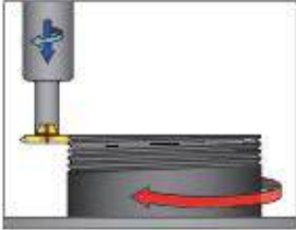
Right Hand Thread-Climb Milling
