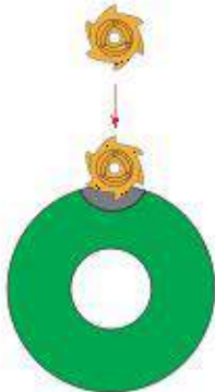
Plunging is not recommended
